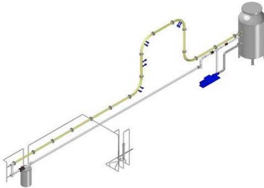
Figure 4: Hilly terrain flow loop is employed in order to investigate wetting in bends (Courtesy of Josh Addis).
