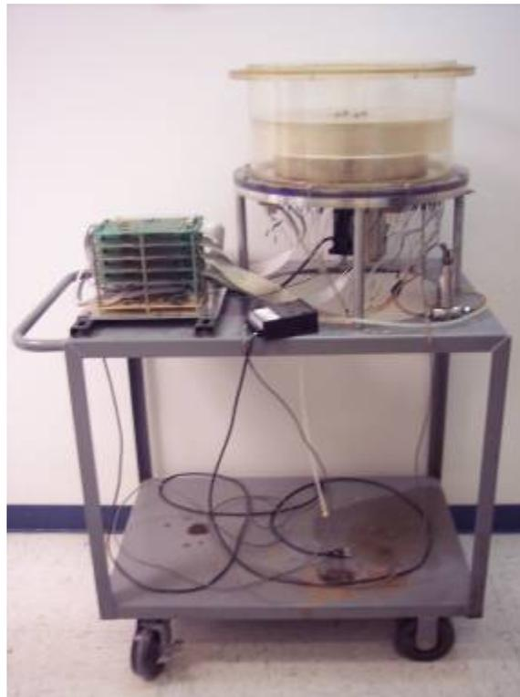
Figure 5. A prototype of a doughnut cell for phase wetting determination (courtesy of Chong Li).
