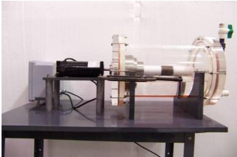
Figure 8: Horizontal rotating cylinder is a benchtop apparatus designed to assess wettability under flowing condition.
