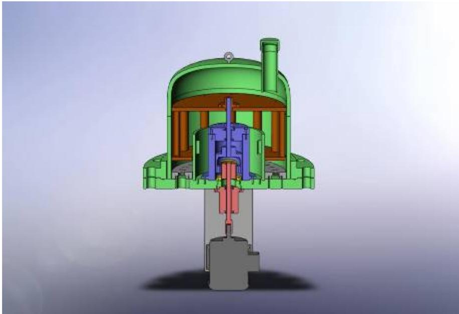
Figure 6: A cross section view of the stainless steel, high temperature, high pressure doughnut cell (Courtesy of Al Schubert).
